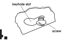
Start screws through neck of each of the four keyhole mounting screw slots marked on the cabinet bottom.
